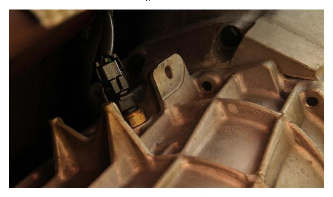
I captured all of the fluid in a drain pan and then measured it to see how much was in there. As it turned out there was about 4.2 quarts. A bit less than the 4.6 called for in the manuals.
